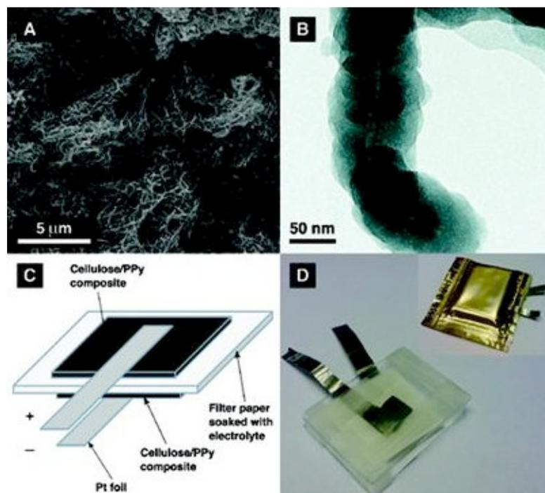
Fig 1. The cellulose-polyppyrol conductive paper composite (a) SEM micrograph taken with a magnification factor of 10 000, (b) TEM image of the cellulose composite fiber, (c) schematic image, and (d) photograph of the composite paper battery cell before and after sealing it into a polymer coated aluminum pouch.
